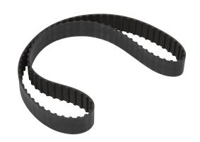
SureMotion timing belt, 3/8in L pitch, 1in wide, 92 tooth, 34.5in pitch length (circumference), neoprene, fiberglass reinforced.
