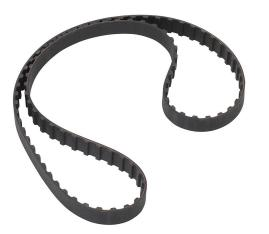
SureMotion timing belt, 3/8in L pitch, 1/2in wide, 92 tooth, 34.5in pitch length (circumference), neoprene, fiberglass reinforced.
