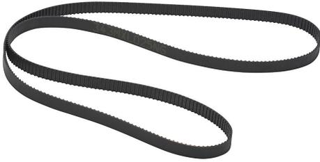
SureMotion timing belt, 0.08in MXL pitch, 1/4in wide, 343 tooth, 27.4in pitch length (circumference), neoprene, fiberglass reinforced. Package of 3.
