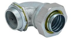
RACO connector, liquid-tight, 90-degree, 1-1/2in trade size, 1-1/2in NPT thread type, zinc electro-plated finish. For use with Liquatite electrical conduit. Sealing washer and locknut included.
