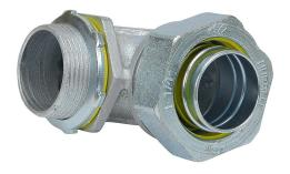
RACO connector, liquid-tight, 90-degree, 1-1/4in trade size, 1-1/4in NPT thread type, zinc electro-plated finish. Package of 10. For use with Liquatite electrical conduit. Sealing washer and locknut included.
