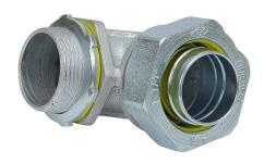
RACO connector, liquid-tight, 90-degree, 1-1/4in trade size, 1-1/4in NPT thread type, zinc electro-plated finish. For use with Liquatite electrical conduit. Sealing washer and locknut included.
