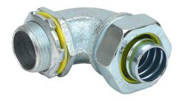
RACO connector, liquid-tight, 90-degree, 3/4in trade size, 3/4in NPT thread type, zinc electro-plated finish. Package of 25. For use with Liquatite electrical conduit. Sealing washer and locknut included.
