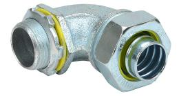
RACO connector, liquid-tight, 90-degree, 3/4in trade size, 3/4in NPT thread type, zinc electro-plated finish. Package of 25. For use with Liquatite electrical conduit. Sealing washer and locknut included.
