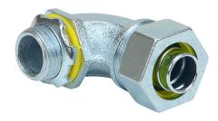
RACO connector, liquid-tight, 90-degree, 1/2in trade size, 1/2in NPT thread type, zinc electro-plated finish. For use with Liquatite electrical conduit. Sealing washer and locknut included.
