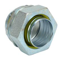
RACO connector, liquid-tight, straight, 2in trade size, 2in NPT thread type, zinc electro-plated finish. For use with Liquatite electrical conduit. Sealing washer and locknut included.
