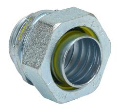
RACO connector, liquid-tight, straight, 1-1/4in trade size, 1-1/4in NPT thread type, zinc electro-plated finish. Package of 10. For use with Liquatite electrical conduit. Sealing washer and locknut included.
