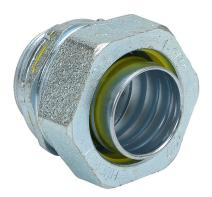
RACO connector, liquid-tight, straight, 1-1/4in trade size, 1-1/4in NPT thread type, zinc electro-plated finish. For use with Liquatite electrical conduit. Sealing washer and locknut included.
