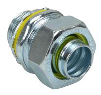
RACO connector, liquid-tight, straight, 3/4in trade size, 3/4in NPT thread type, zinc electro-plated finish. For use with Liquatite electrical conduit. Sealing washer and locknut included.
