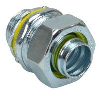
RACO connector, liquid-tight, straight, 3/4in trade size, 3/4in NPT thread type, zinc electro-plated finish. For use with Liquatite electrical conduit. Sealing washer and locknut included.
