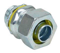
RACO connector, liquid-tight, straight, 1/2in trade size, 1/2in NPT thread type, zinc electro-plated finish. Package of 50. For use with Liquatite electrical conduit. Sealing washer and locknut included.
