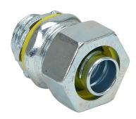
RACO connector, liquid-tight, straight, 1/2in trade size, 1/2in NPT thread type, zinc electro-plated finish. For use with Liquatite electrical conduit. Sealing washer and locknut included.
