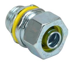
RACO connector, liquid-tight, straight, 3/8in trade size, 1/2in NPT thread type, zinc electro-plated finish. Package of 50. For use with Liquatite electrical conduit. Sealing washer and locknut included.
