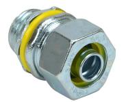
RACO connector, liquid-tight, straight, 3/8in trade size, 1/2in NPT thread type, zinc electro-plated finish. For use with Liquatite electrical conduit. Sealing washer and locknut included.
