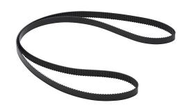
SureMotion timing belt, 0.08in MXL pitch, 1/4in wide, 330 tooth, 26.4in pitch length (circumference), polyurethane, polyester reinforced. Package of 3.
