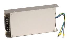
AutomationDirect EMI input filter, 230 VAC, 1-phase, 32A, panel mount, EMI/RFI filtering, drive rated, standard performance, screw terminals and ring terminals. For use with 1-phase AC drives.
