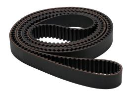
SureMotion timing belt, 8mm 8M pitch, 30mm wide, 410 tooth, 3280mm pitch length (circumference), neoprene, fiberglass reinforced.
