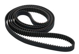
SureMotion timing belt, 8mm 8M pitch, 20mm wide, 410 tooth, 3280mm pitch length (circumference), neoprene, fiberglass reinforced.
