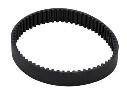
SureMotion timing belt, 5mm 5M pitch, 15mm wide, 65 tooth, 325mm pitch length (circumference), neoprene, fiberglass reinforced.
