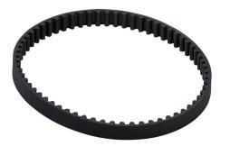
SureMotion timing belt, 5mm 5M pitch, 9mm wide, 65 tooth, 325mm pitch length (circumference), neoprene, fiberglass reinforced.
