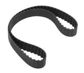
SureMotion timing belt, 3/8in L pitch, 1in wide, 86 tooth, 32.2in pitch length (circumference), neoprene, fiberglass reinforced.
