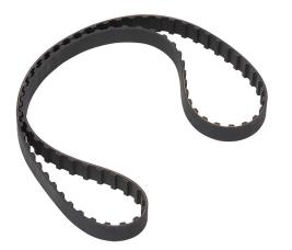
SureMotion timing belt, 3/8in L pitch, 1/2in wide, 86 tooth, 32.2in pitch length (circumference), neoprene, fiberglass reinforced.
