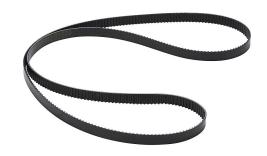
SureMotion timing belt, 0.08in MXL pitch, 1/4in wide, 320 tooth, 25.6in pitch length (circumference), polyurethane, polyester reinforced. Package of 3.
