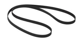
SureMotion timing belt, 0.08in MXL pitch, 1/4in wide, 320 tooth, 25.6in pitch length (circumference), neoprene, fiberglass reinforced. Package of 3.
