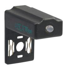
Murrelektronik solenoid valve surge suppressor, Zener diode, 18-30 VAC/VDC, 1-phase, 0-60Hz, 100W, vertical mount. For use with 9.4mm DIN style Form C plug.
