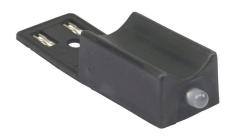
Murrelektronik solenoid valve surge suppressor, resistorcapacitor, 95-132 VA/VDC, 1-phase, 0-60Hz, 10W, horizontal mount. For use with 11mm DIN style Form B plug.
