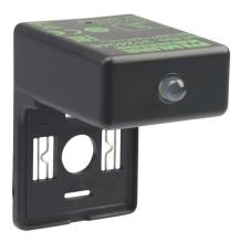
Murrelektronik solenoid valve surge suppressor, varistor, 48-130 VAC/VDC, 1-phase, 0-60Hz, 100W, vertical mount. For use with 18mm DIN style Form A plug.
