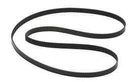
SureMotion timing belt, 0.08in MXL pitch, 1/4in wide, 310 tooth, 24.8in pitch length (circumference), polyurethane, polyester reinforced. Package of 3.
