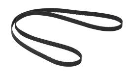
SureMotion timing belt, 0.08in MXL pitch, 1/4in wide, 310 tooth, 24.8in pitch length (circumference), neoprene, fiberglass reinforced. Package of 3.
