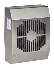
Seifert SoliTherm thermoelectric cooler, 170 BTU/H, 24 VDC operating voltage, 304 stainless steel housing, filter-free, recessed mount. For use with NEMA 4/4X/12 enclosures.
