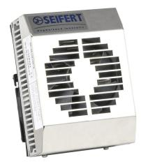
Seifert SoliTherm thermoelectric cooler, 100 BTU/H, 24 VDC operating voltage, 304 stainless steel housing, filter-free, recessed mount. For use with NEMA 4/4X/12 enclosures.
