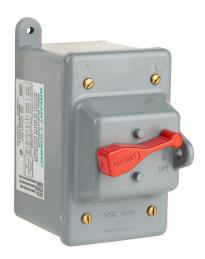
Bryant manual motor controller, enclosed, 30A, 600 VAC, 3-pole, 20hp, wall mount, thermoplastic housing, NEMA 3R, UL 508 rated.
