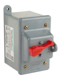
Bryant manual motor controller, enclosed, 30A, 600 VAC, 2-pole, 15hp, wall mount, thermoplastic housing, NEMA 3R, UL 508 rated.
