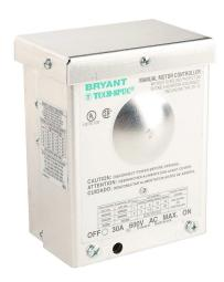
Bryant manual motor controller, enclosed, 30A, 600 VAC, 2-pole, 15hp, wall mount, die-cast aluminum housing, NEMA 3R, UL 508 rated.
