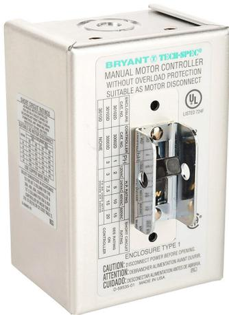
Bryant manual motor controller, enclosed, 30A, 600 VAC, 3-pole, 20hp, wall mount, aluminum housing, NEMA 1, UL 508 rated.
