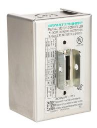
Bryant enclosure without manual motor controller, NEMA 1. Lockout/tagout hardware and switch mounting screws included. Use as a replacement enclosure for 30102D and 30103D or use with switch 30002D or switch 30003D to make a 30A manual motor controller.
