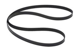
SureMotion timing belt, 0.08in MXL pitch, 1/4in wide, 300 tooth, 24in pitch length (circumference), polyurethane, polyester reinforced. Package of 3.
