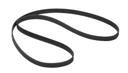
SureMotion timing belt, 0.08in MXL pitch, 1/4in wide, 300 tooth, 24in pitch length (circumference), neoprene, fiberglass reinforced. Package of 3.
