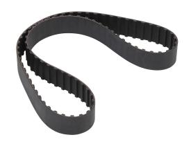
SureMotion timing belt, 3/8in L pitch, 1in wide, 80 tooth, 30in pitch length (circumference), neoprene, fiberglass reinforced.
