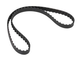
SureMotion timing belt, 3/8in L pitch, 1/2in wide, 80 tooth, 30in pitch length (circumference), neoprene, fiberglass reinforced.
