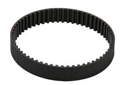
SureMotion timing belt, 5mm 5M pitch, 15mm wide, 60 tooth, 300mm pitch length (circumference), neoprene, fiberglass reinforced.
