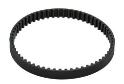
SureMotion timing belt, 5mm 5M pitch, 9mm wide, 60 tooth, 300mm pitch length (circumference), neoprene, fiberglass reinforced.
