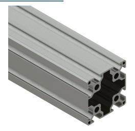
SureFrame 30 Series standard T-slotted rail, silver, 6063-T6 anodized aluminum alloy, cut to length, 60 x 60mm profile, slot size 8.
