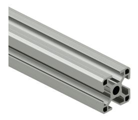
SureFrame 30 Series standard T-slotted rail, silver, 6063-T6 anodized aluminum alloy, cut to length, 30 x 30mm profile, slot size 8.
