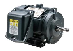
Toshiba SD premium efficiency AC induction motor, high-performance inverter duty and severe duty, 3/4hp, 3-phase, 230/460 VAC, 1200rpm, TEFC, NEMA 56 frame, cast iron, rigid base mount.
