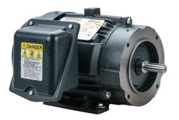
Toshiba SD premium efficiency AC induction motor, highperformance inverter duty and severe duty, 3/4hp, 3-phase, 230/460 VAC, 1800rpm, TEFC, NEMA 56C frame, cast iron, C-face/ rigid base mount.
