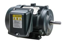
Toshiba SD premium efficiency AC induction motor, high-performance inverter duty and severe duty, 3/4hp, 3-phase, 230/460 VAC, 1800rpm, TEFC, NEMA 56 frame, cast iron, rigid base mount.
