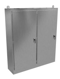
Hammond disconnect enclosure, NEMA 3R/4/4X/12/13, right flange, 90 x 79 x 20in (HxWxD), freestanding, 304 stainless steel, #4 brush finish, 2-door, 3-point padlocking handle, subpanel included.
